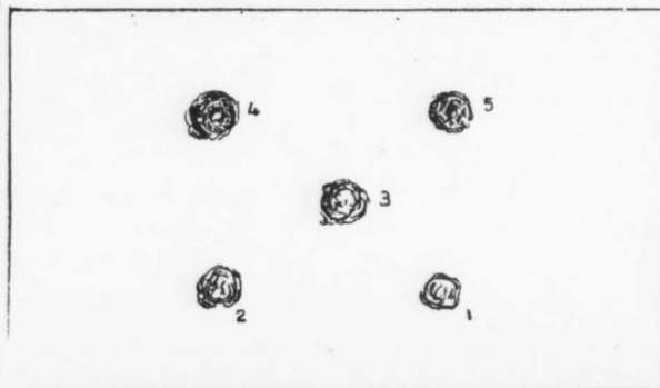
FIG. 10. Schneider steel armour-plate for the Spanish cruiser Cataluna , 250 millimetres (9.84 in.) thick. Tested June 14, 1897. Rounds 1, 2, 3; Holtzer projectile, 5.90 in. in diameter, weight 99 lb.; velocity, 1900 ft. to 1918 ft.
